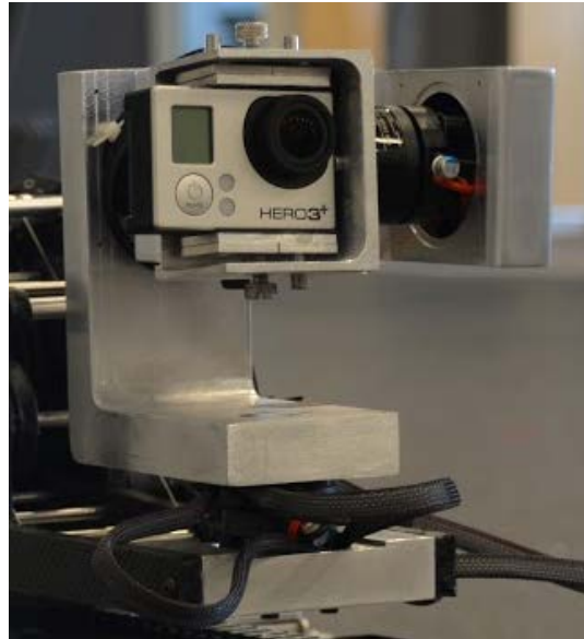
Figure 5.18: Manufactured Gimbal and Camera Holder
