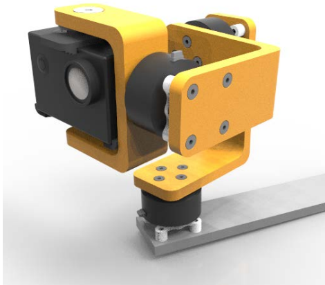
Figure 5.16: Rendering of first CAD of gimbal with solid arms
