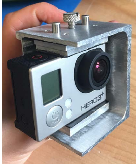
Figure 5.20: Finished camera holder
